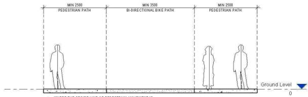
WHERE THE DESIRE LINE OF PEDESTRAIN MOVEMENT IS ALONG BOTH SIDES OF THE CORRIDOR
